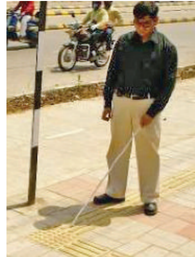
Tactile paving on footpath (Source: UTTIPEC Streetscaping Guidelines 2010)
